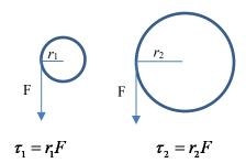
Want to maximize the torque on the screw, so use a wider handle (increase r).
