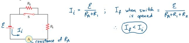
A circuit is comprised of two rectangular loops, one on top of the other. The bottom loop contains a battery on the left side with the positive terminal on the bottom, an ammeter on the bottom side, a resistor  $R_1$  on the right side, and a closed switch on the top side. The top loop contains a resistor  $R_2$  on the top side and a closed switch on the bottom side which is also the top side of the bottom loop. When the switch is opened, the reading on the ammeter...
