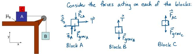
Given the following values, calculate the minimum required mass of block C such that block A does not slide on the table top. To receive full marks, you must include a diagram showing the physical situation and your choice of coordinate system.  $m_A = 5.81$  kg;  $m_B = 3.04$  kg;  $\mu_s = 0.211$  ANS:  $m_C = 8.6$  kg
