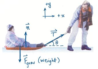
Note that the net force in the vertical direction is zero.  $\therefore \Sigma F_y = 0$  $\therefore + n + T \sin 0 - F_{grav} = 0$  $\therefore n = F_{grav} - T \sin 0$  $\therefore n < F_{grav}$
