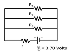
(a) Calculate the current flowing through the internal resistance r. (5 marks)
