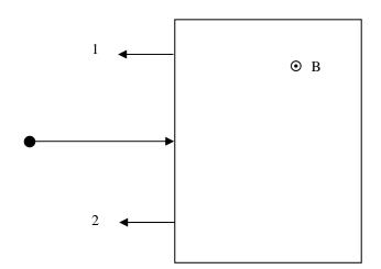
When the alpha particle leaves the region of magnetic field it is moving opposite to its original direction.
