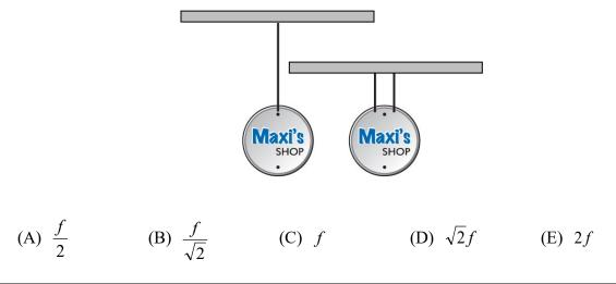
Let  $L_1$  be the original length of the wire. At the fundamental mode of resonance, the length of the wire corresponds to  $\frac{1}{2}$  the wavelength because there will be a node at each end of the wire.
