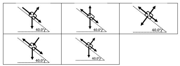
B10. Let *a* represent the magnitude of the acceleration of the two crates. Which one of the following is the correct formula for the magnitude of the normal force of the incline on the 5.00-kg crate?
