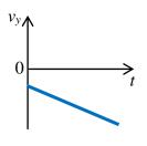
The +y direction was chosen to be up. The ball moves downward throughout its motion, so  $v_y$  is negative. Since air resistance can be ignored, the acceleration is constant and downward, so  $v_y$  vs. time will be linear with a negative slope, and the value of  $v_y$  will become increasingly negative.
