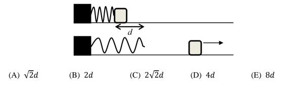
Since the surface is frictionless, mechanical energy is conserved.  $KE_i + PE_i = KE_f + PE_f \Rightarrow 0 + \frac{1}{2}kd^2 = \frac{1}{2}mv_1^2 + 0 \Rightarrow v_1 = d\sqrt{k}$  That is, the speed is directly proportional to the compression of the spring (*k* is a constant). So to obtain double the speed, the compression must be doubled. Option (B) is correct.
