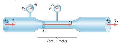
(a) The pressure difference,  $P_2 - P_1$ , between the two sections of pipe, is measured to be  $1.20 \times 10^2$  Pa. Calculate  $v_2$ , the flow speed in the main pipe. *Hint: Start by deriving an expression relating*  $v_1$  *to*  $v_2$ . (7 marks)
