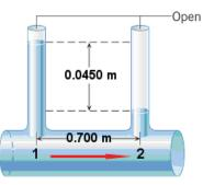
(a) Calculate the pressure difference,  $P_1 - P_2$ , between locations 1 and 2. (3 marks)
