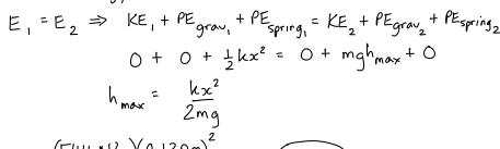
$$h_{\text{max}} = \frac{(544 \text{ N/m})(0.120 \text{ m})^2}{2(20.0 \times 10^{-3} \text{ kg})(9.80 \text{ m/s}^2)} = (20.0 \text{ m})$$
