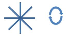
(a) Model the spider as a set of 8 identical thin rods, each of length 1.00 cm and mass  $0.200 \times 10^{-3}$  kg, with all the rods arranged radially around the axis of rotation. Calculate the rotational inertia, *I*, of the spider. (4 marks)
