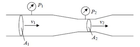
(a) Derive an expression for  $v_2$ , the speed where the cross-sectional area is  $A_2$ , in terms of  $v_1$ ,  $A_1$ , and  $A_2$ . (3 marks)
