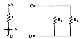
(a) Calculate the equivalent resistance between the terminals C and D of the resistor network.
