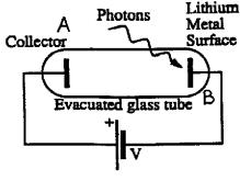
$$KE_{max} = \frac{hc}{\lambda} - W_0 = \frac{(4.14 \times 10^{-15} \text{eV} \cdot \text{s})(3.00 \times 10^8 \text{m/s})}{450 \times 10^{-9} \text{ m}} - 2.30 \text{eV}$$
