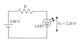
(a) Calculate the current flowing in the circuit.
