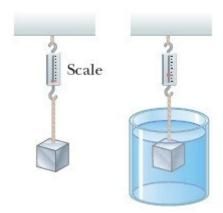
At the left, the figure shows a vertical spring scale. The top of the scale has a hook attached to the ceiling. The bottom of the scale has a hook attached to a rope. The rope hangs down and is attached to the object that hangs from the rope. At the right, the figure shows the same scale, but now the object is submerged in a tank of water. The reading on the scale at the right is less than the reading on the scale at the left.  $2350 \text{ kg/m}^3$
