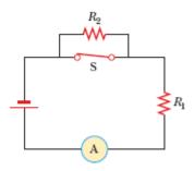
A circuit is comprised of two rectangular loops, one on top of the other. The bottom loop contains a battery on the left side with the positive terminal on the bottom, an ammeter on the bottom side, a resistor  $R_1$  on the right side, and a closed switch on the top side. The top loop contains a resistor  $R_2$  on the top side and a closed switch on the bottom side which is also the top side of the bottom loop.
