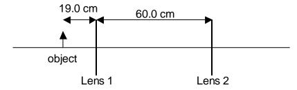
(a) Determine the location of the final image relative to lens 2.
