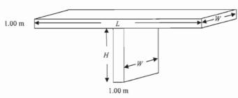
Show that the pressure on the bottom of the concrete support column is independent of the width W. For L = H = 100 m, calculate the compression stress, in Pa, at the bottom of the column. Use 2400 kg/m<sup>3</sup> for the density of concrete. (3 marks)
