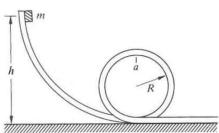
(a) Calculate the speed of the object at the instant when it just barely loses contact with the track at the top of the loop. (4 marks)
