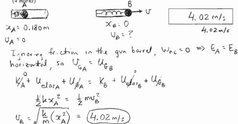
(b) Calculate the speed of the ball in the instant before it hits the ground, a distance of 1.70 m below the release point (where it left the gun)? (3 marks) If you did not obtain an
