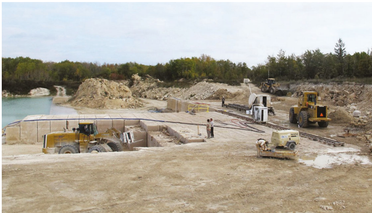
Gillis Quarries Ltd. in operation, showing front-end loaders, sawn grid, and circular and belt saws.
