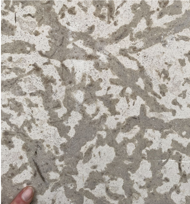
Surface sawn parallel to bedding showing bioclastic packstone (light) with dolomite mottles (dark) related to burrows.
