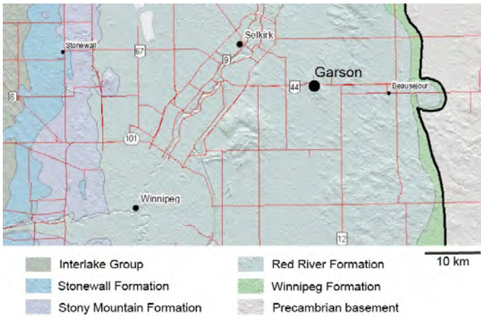
Figure 5. Geological map of the Winnipeg area, southern Manitoba. Adapted from Nicolas et al. (2010).
